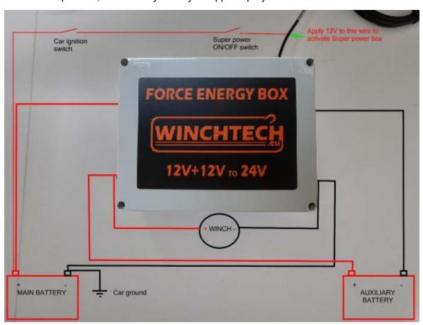
The Force Energy box is connected between your existing vehicle battery and a second auxiliary battery. The auxiliary battery should not be grounded or connected to anything else, just the two heavy cables from the Force Energy Box.
